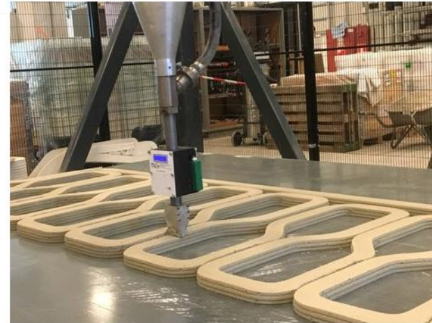
The team printed used a customized printer to lay down layers of concrete, one after another, and include steel reinforcement at the same time. Image credit: Eindhoven University of Technology.
